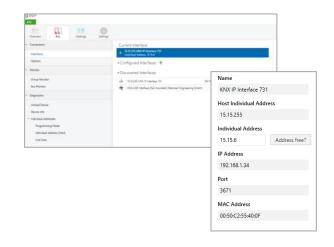
The individual KNX device address and the individual addresses for additional tunneling connections can be changed within the ETS project after the device has been added to the project.
