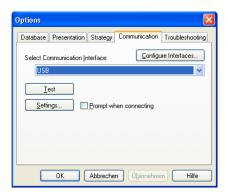
After clicking the button "Configure Interfaces" the ETS Connection Manager opens. You have to create a new connection type EIBnet/IP. The ETS begins with the automatic search of all KNXnet/IP devices. All found devices are displayed. Select the required device.
